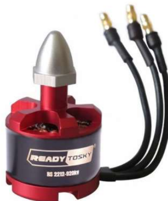
Slika 5.4 ReadytoSky RS 2212 – 920 KV BLDC motor
