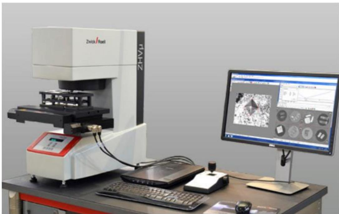
**Slika 38:** Zwick Roell ZHV $\mu$  Micro Vickers Hardness Tester [37]
