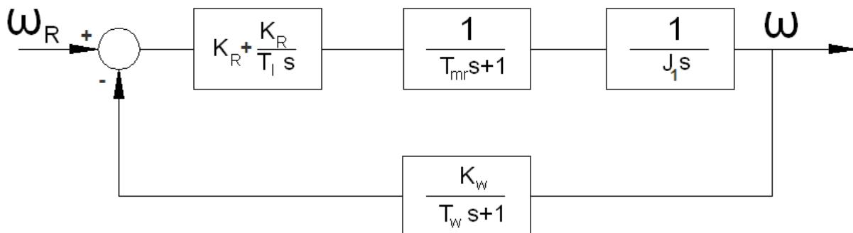
Slika 4.8 Blok shema PI regulatora u petlji momenta
