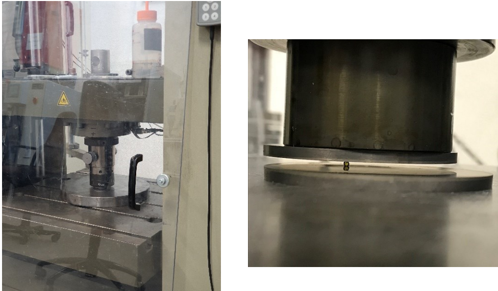
Figure 44: Zwick/Roell force sensor 250kN with single diamond particle sandwiched between PCD plates
