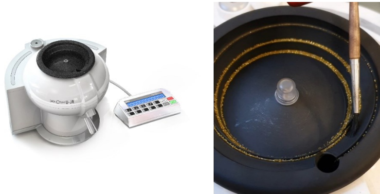
Figure 20: Particle counting machine used in experiments
