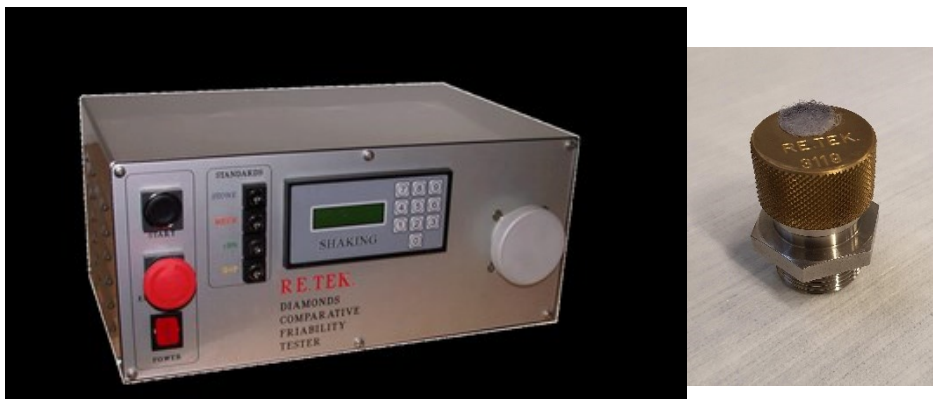
Figure 31: Friability tester from ReTek company with capsule [23]
