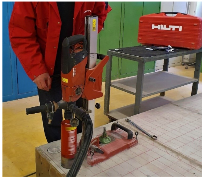
Figure 54: Testing setup with DD150 drill, on drill stand
