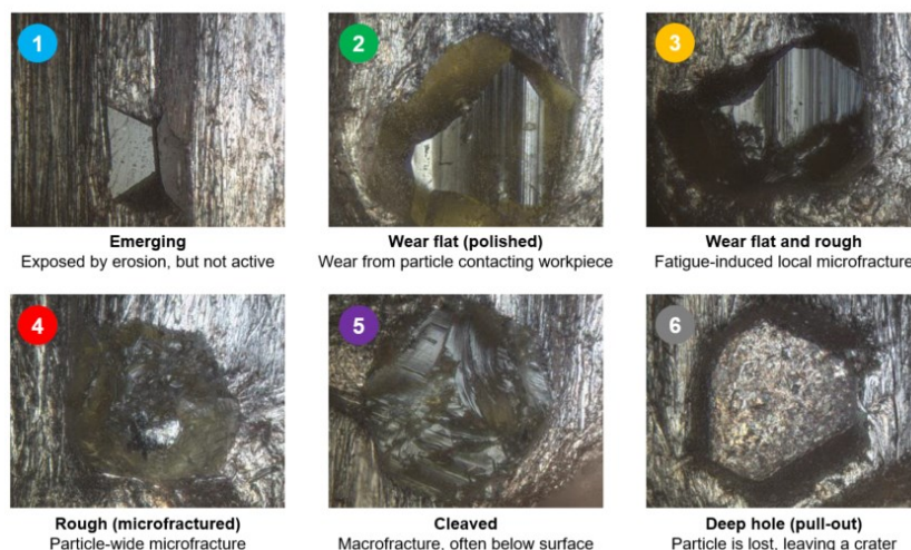
Figure 34: Diamond wear states and particle lifecycle
