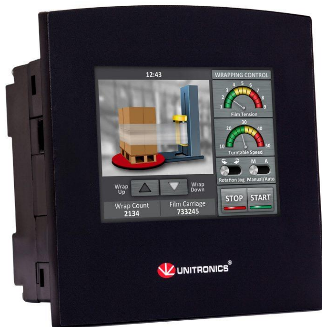
Slika 55. PLC – Unitronics Samba [27]
