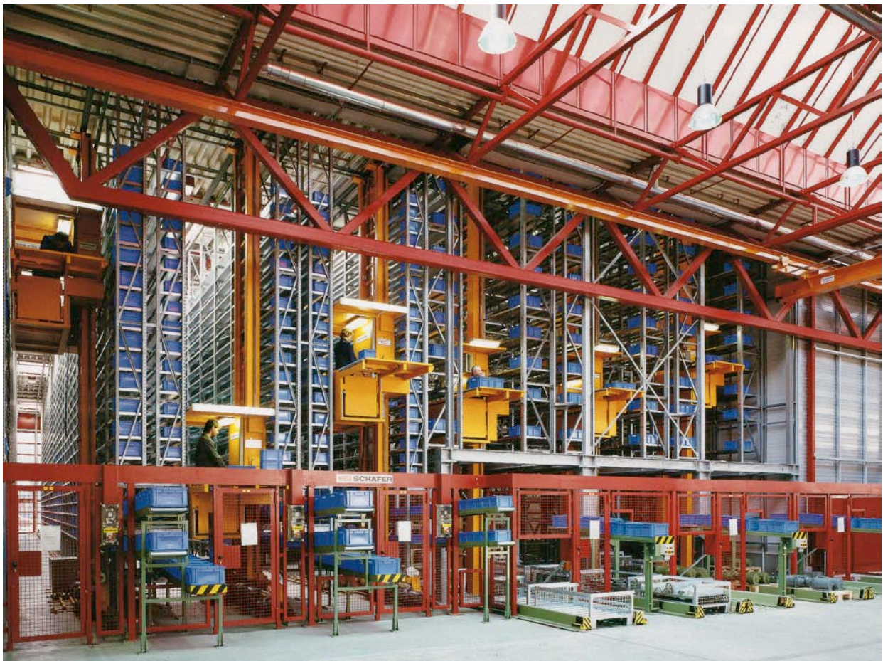
Slika 25. Person on board AS/RS
