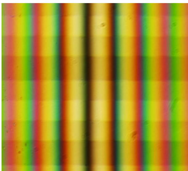
Slika 6.18 Etalon nazivne dubine brazde 50 nm. Interferogram primarne strukture Si/SiO<sub>2</sub>
