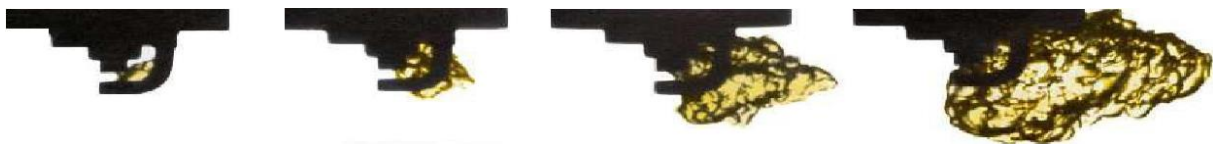
Figure 13. Visualization of the early flame kernel growth from the experiment [55] indicating the effects of local bulk flow and turbulence in the vicinity of the spark plug.
