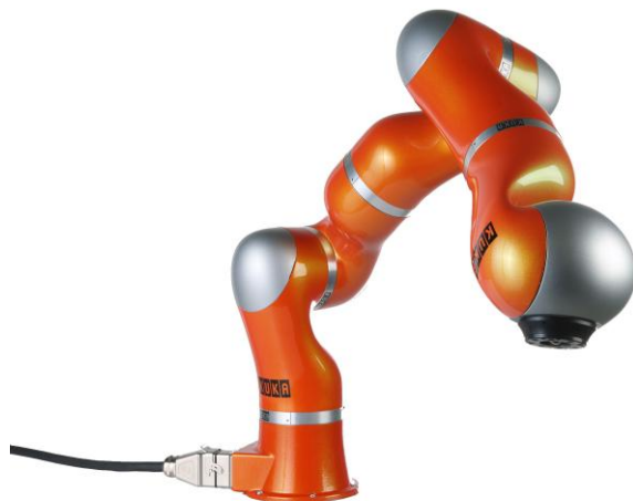
Slika 2.4. Kuka robotska ruka – LWR4+ (lightweight robot).
