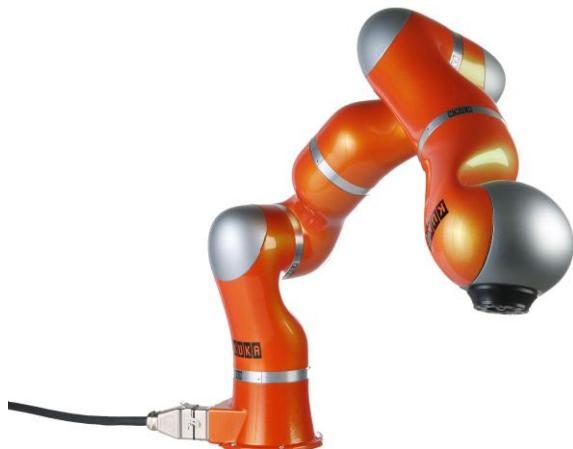
Slika 2.4. Kuka robotska ruka – LWR4+ (lightweight robot).
