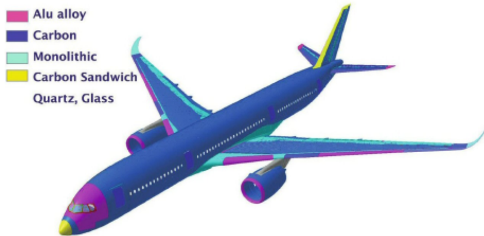
Figure 1.2: Airbus A350 structural materials [McConnell, 2011].
