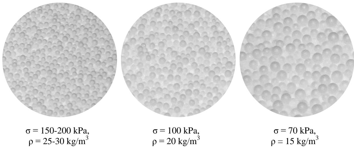
**Sl.- 23.** Ilustrirani prikaz predekspandiranih zrna polistirena promjera: a)  $\varnothing = 2,5 - 3 \text{ mm}$ , b)  $\varnothing = 3 \text{ mm}$  i c)  $\varnothing = 4 \text{ mm}$  [66].
