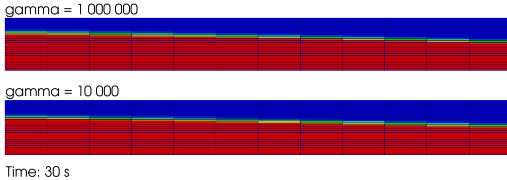
Figure 6.12: Interface resolution at the end of simulation ( t = 30 s) for different stabilisation parameters, \gamma . The interface is almost identically smeared across two cells for both cases, controlled by a width parameter \epsilon = 0.004 . Only part of the domain is shown: x \in [29, 31] , y \in [-0.1, 0.1] for clarity.
