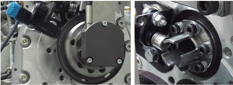
Figure 49. Left: Hall sensor on the crankshaft; Right: Hall sensor on the camshaft
