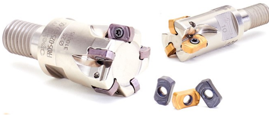
Slika 54. Glodaća glava (fourworks) za High feed milling [10]
