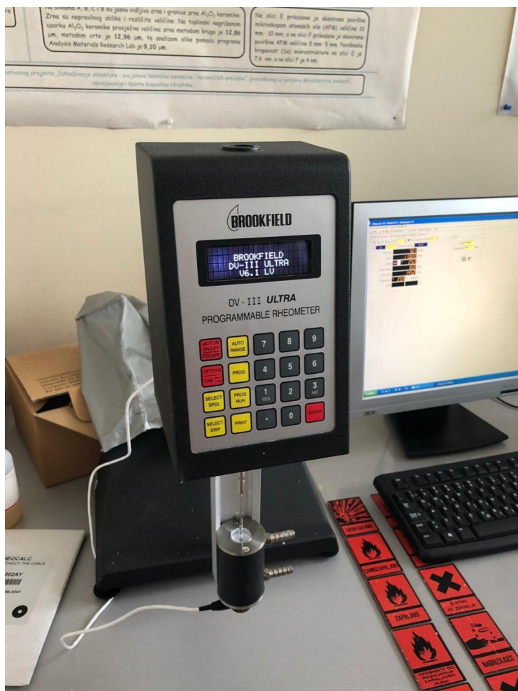
Slika 14. Reometar Brookfield DV-III Ultra (Brookfield Engineering Laboratories, Inc., SAD)
