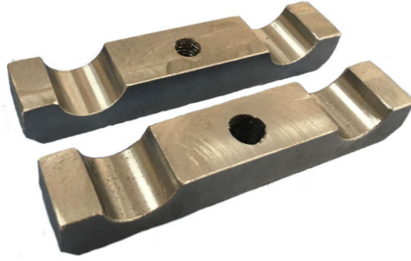
Figure 3 – Etalons for sets 1 (two pairs were manufactured for each of the sets)
