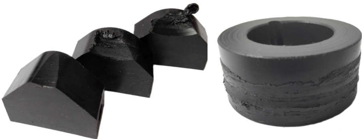
Figure 10 – Damaged static (left) and rotating (right) specimens
