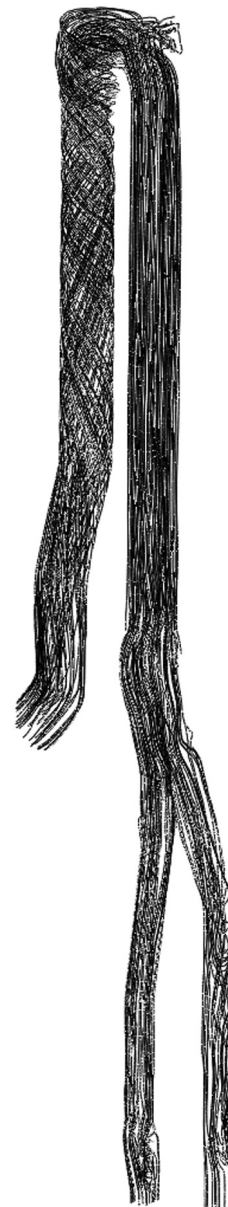
Fig. 2. Flow streamlines inside the calculated calciner.
