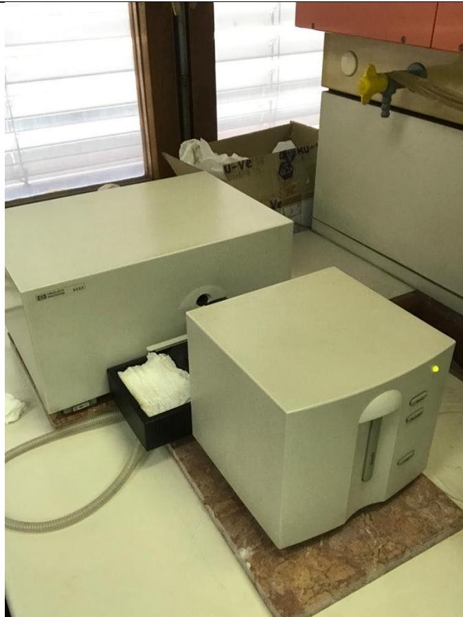
**Slika 6. Spektrofotometar Hewlett Packard, model 8453 (Hewlett Packard, SAD)**
