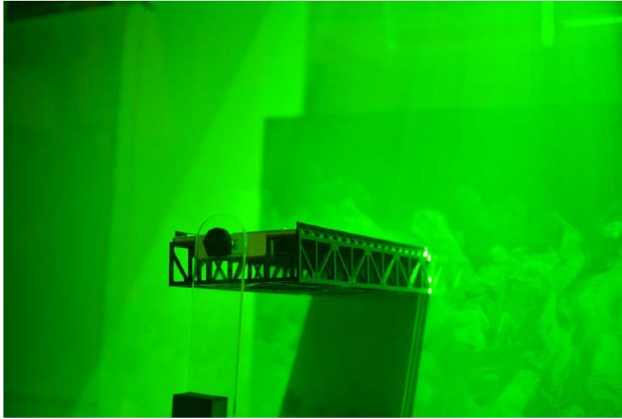
Figure 15: Seeding particles around the bridge-deck section model illuminated by laser.
