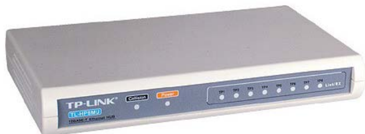
4.12. Ethernet Hub TP-Link TL-HP8M
