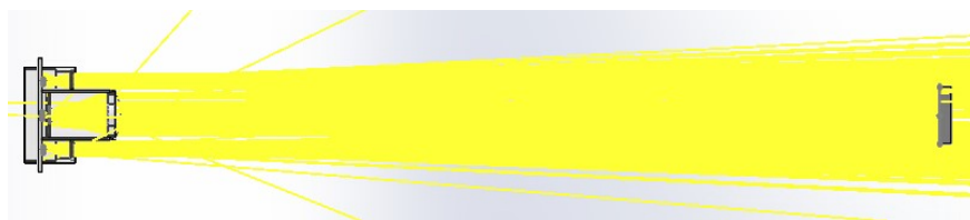
Fig. 1 TF_mini optical simulation of the optical path
