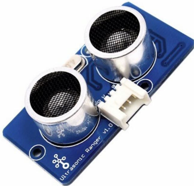
This Grove - Ultrasonic ranger is a non-contact distance measurement module which works at 40KHz. When we provide a pulse trigger signal with more than 10uS through singal pin, the Grove\_Ultrasonic\_Ranger will issue 8 cycles of 40kHz cycle level and detect the echo. The pulse width of the echo signal is proportional to the measured distance. Here is the formula: Distance = echo signal high time \* Sound speed (340M/S)/2. Grove\_Ultrasonic\_Ranger's trig and echo singal share 1 SIG pin.
