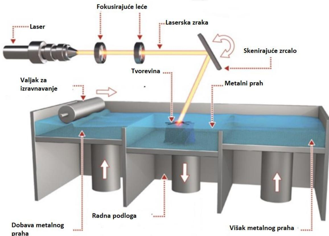
Slika 7. Shema SLM/DMLS 3D printera metal [13]
