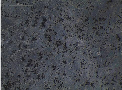
Micrograph showing a dark surface with a significant increase in light-colored, irregular spots and some larger, darker patches, indicating surface degradation. A scale bar of 0.5 mm is visible at the top left.           |
