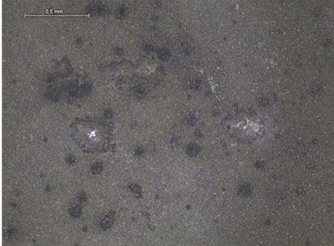
Micrograph showing a dark surface with a significant increase in light-colored spots and some larger, darker patches, indicating surface degradation. A scale bar of 0.5 mm is visible at the top left.                    |
