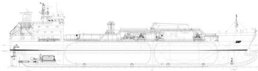
Slika 8.1. Opći plan LPG broda  $6500 \text{ m}^3$
