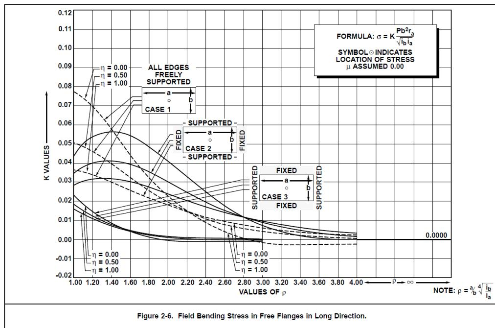
Figure 2-6. Field Bending Stress in Free Flanges in Long Direction.
