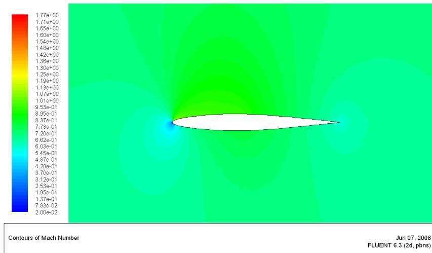
Slika 5.25:  $M_\infty=0.7$ ,  $\alpha = 2^\circ$ ,  $M_{max}=1.062$
