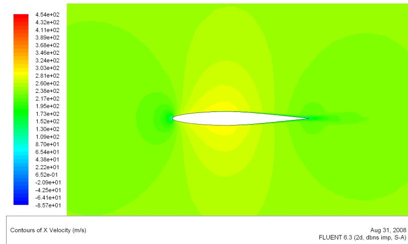
Slika 5.41: Konture  $V_x$  komponente brzine,  $M_\infty=0.7$ ,  $\alpha = 0^\circ$
