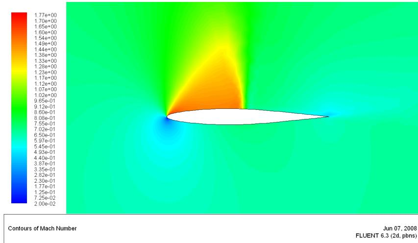
Slika 5.27:  $M_{\infty}=0.7$ ,  $\alpha = 6^\circ$ ,  $M_{max}=1.611$
