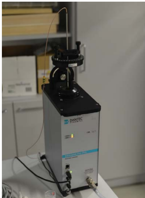
Figure 3.8 Dantec Dynamics StreamLine Pro Calibrator for hot-wire calibration, Marušić [20]
