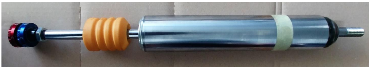
Slika 117. Amortizer TEIN Super racing
