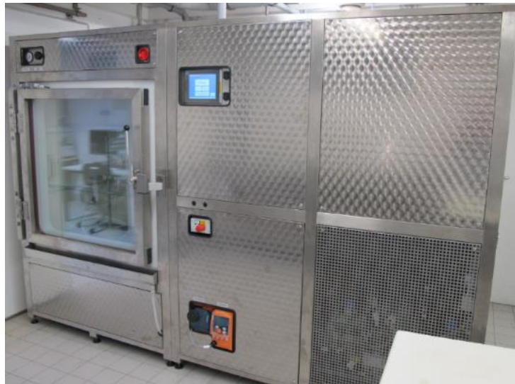
Figure 8. “HKS 700” climatic test chamber
