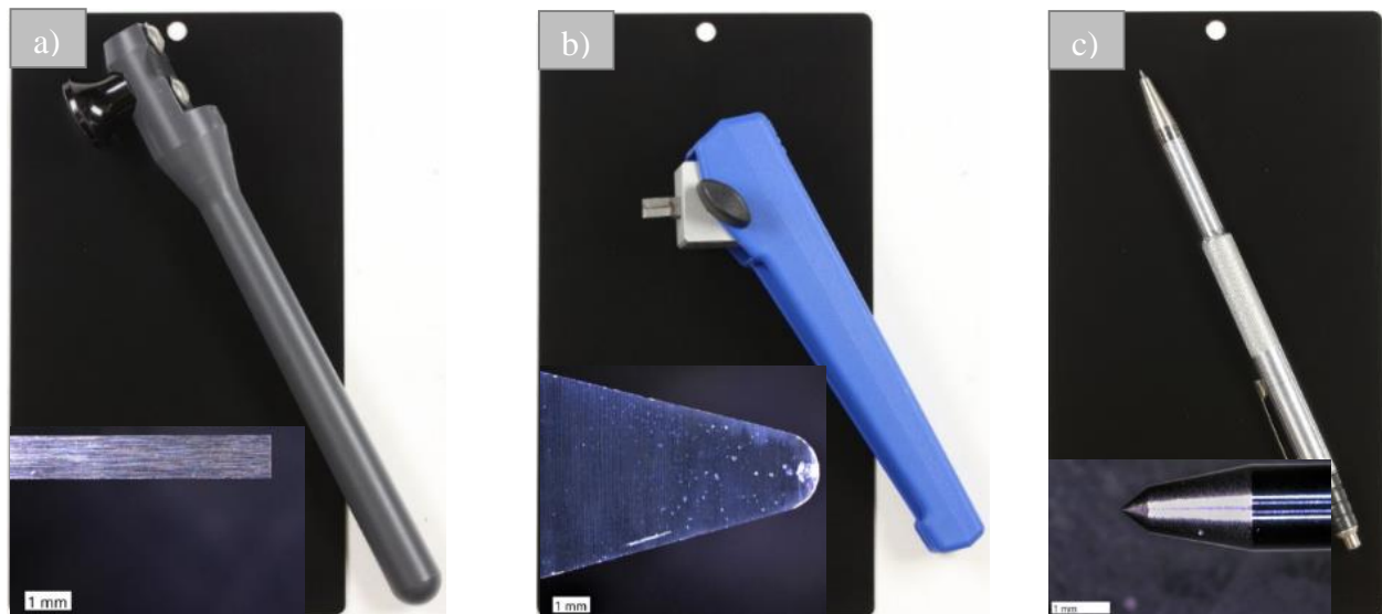
Figure 17. Scribing tools with respective scribing tips a) Sikkens b) Clemen c) Van Laar
