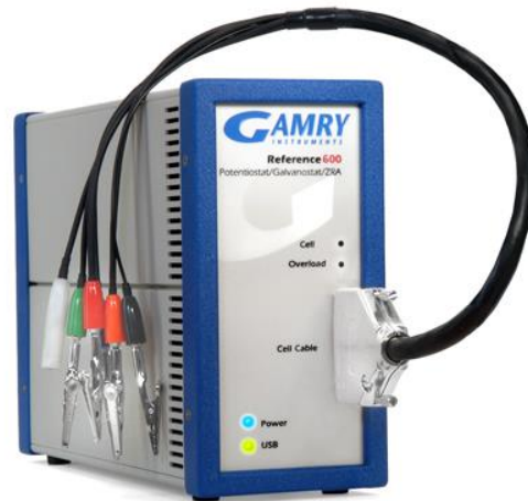
Figure 56. „Gamry Reference 600“ potentiostat [40]
