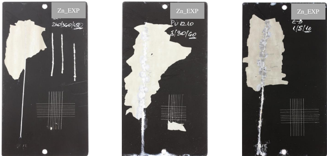
Figure 59. Zn_EXP specimens with poor coating adhesion after 480 hours of CH, 60 cycles of PV 1210, and 10 cycles of Cycle –B test
