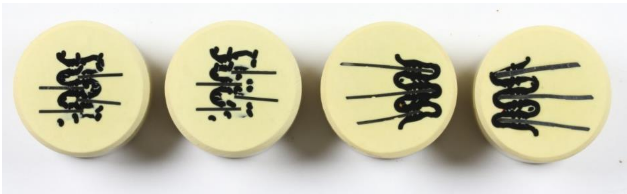
Figure 11. Embedded specimen samples for optical microscopy
