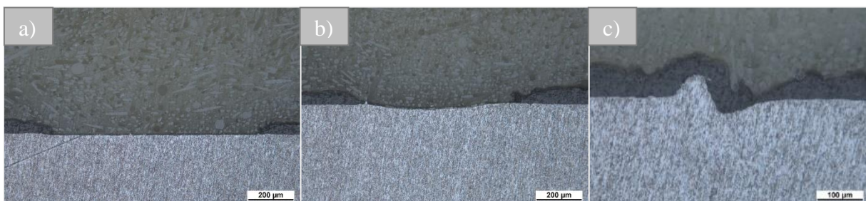
Figure 19. Cross section samples of the scribe lines a) Sikkens b) Clemen c) van Laar
