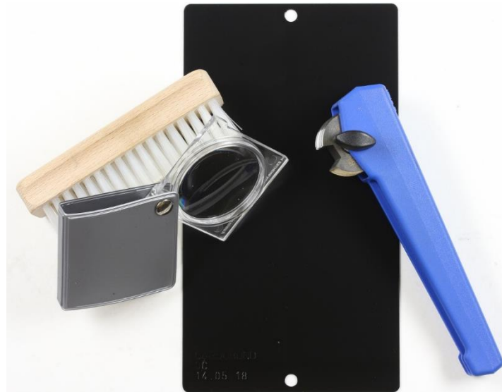
Figure 25. Cross cut tool with brush and magnifying glass from „Erichsen“
