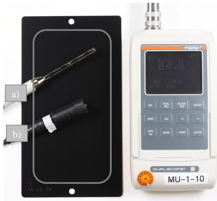
Figure 30. „Dualscope MP 40“coating thickness measuring device with a) ferrous substrate probe b) aluminium substrate probe
