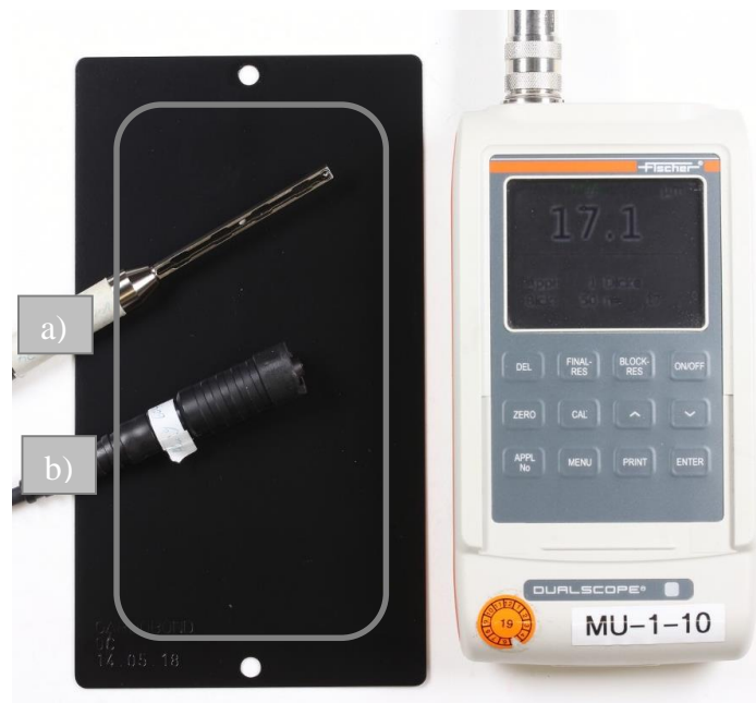
Figure 30. „Dualscope MP 40“coating thickness measuring device with a) ferrous substrate probe b) aluminium substrate probe
