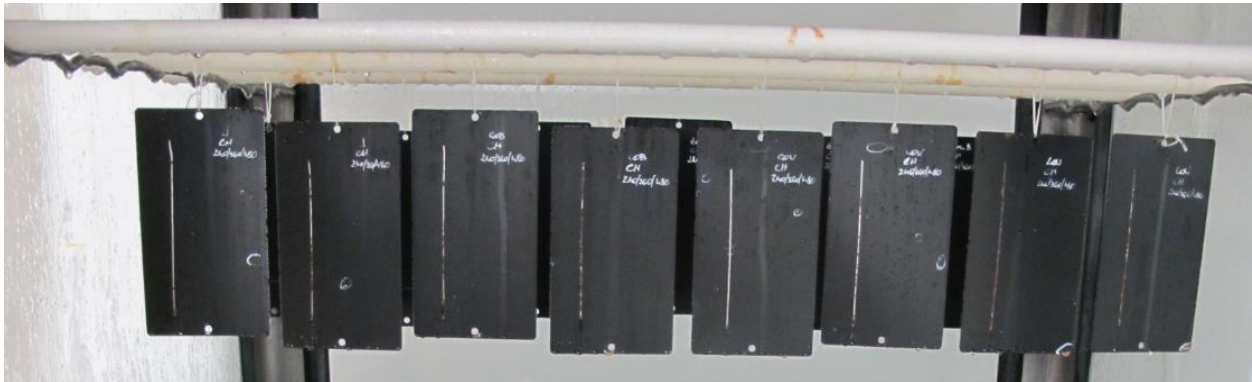
Figure 35. Placement of the specimens in the CH test chamber
