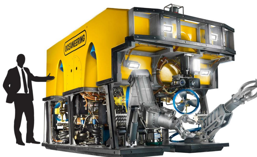
Slika 2.6 Oceanering Millennium Plus Work class ROV (165kW)
