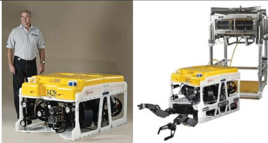
**Slika 2.7 SAAB Seaeye Cougar-XT Medium sized ROV (30kW)**
