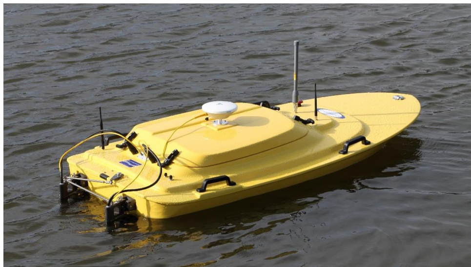
Slika 2.2 Teledyne Marine Z-boat ASV
