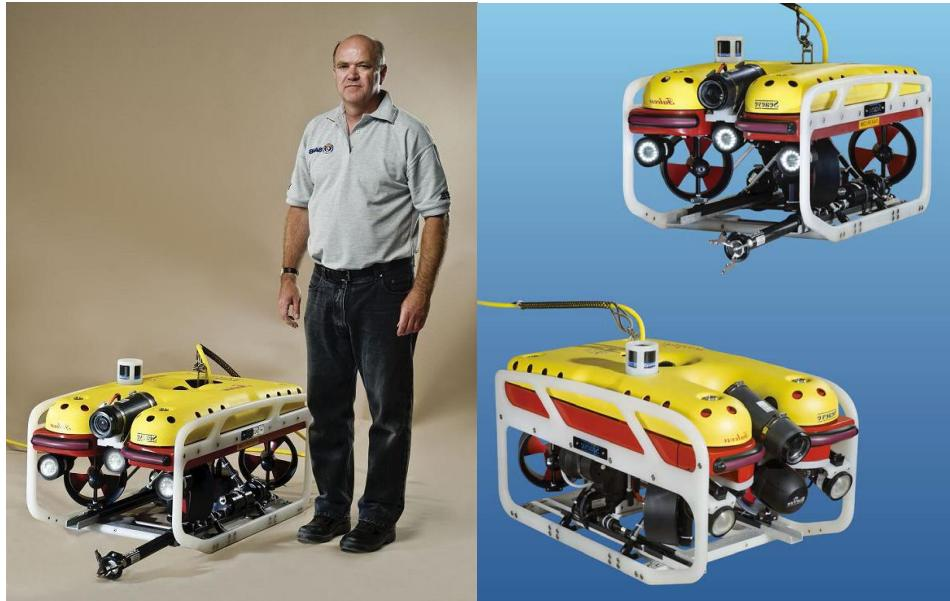
**Slika 2.8 SAAB Seaeye Falcon Observation class ROV (100kg)**
