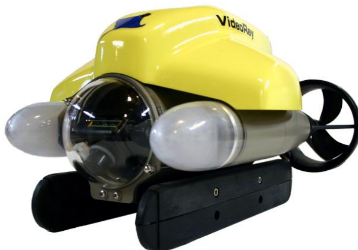
Slika 2.9 VideoRay PRO4 Observation class ROV (5Kg)
