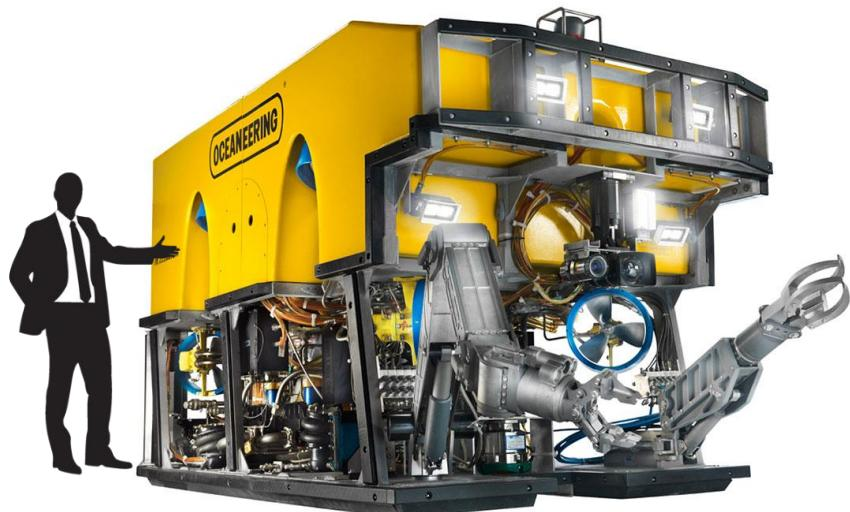
**Slika 2.6 Oceaneering Millennium Plus Work class ROV (165kW)**
