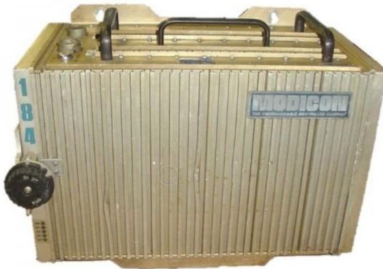
Slika 2. PLC model Modicon 184 [6]
