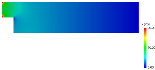
Figure 5.1.20: Backward facing step BF pressure field visualization, laminar simulation
