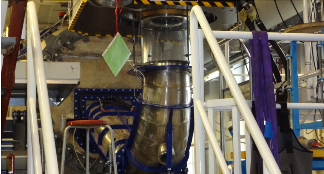
Figure 5.3.1: Test rig of the model Francis turbine/pump-turbine [19]
