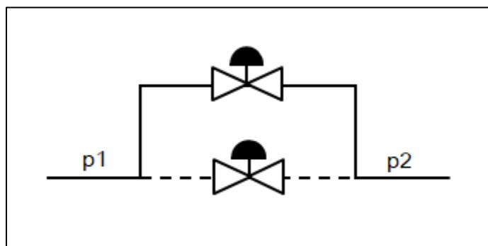
Slika 2.5 Shema mimovodog cjevovoda
