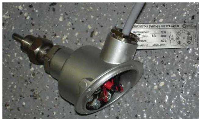
Slika 8: Temperaturna sonda Pt-100
