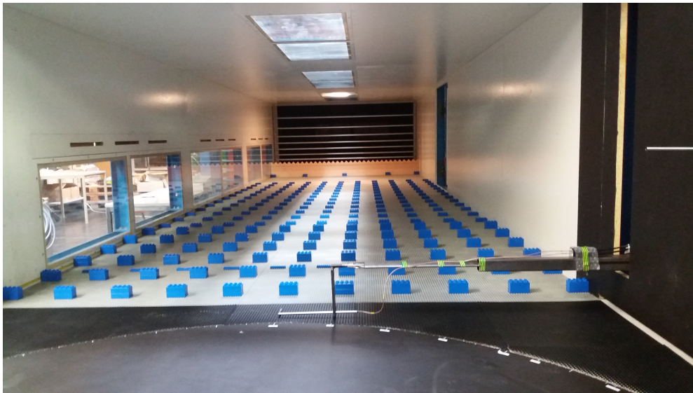
Figure 3.15: Hot-wire probe mounted on a traverse support in the IFMHT-GUT wind tunnel [37]
