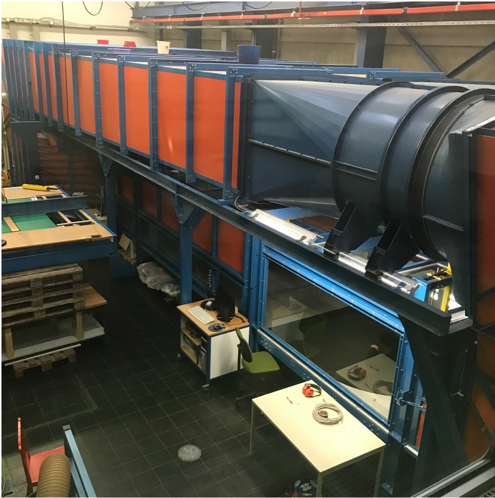
Figure 3.1: Boundary layer wind tunnel at the IFMHT
