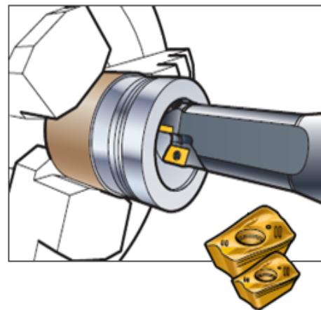
d) Koaksijalno glodanje (Circular interpolation in helix)
