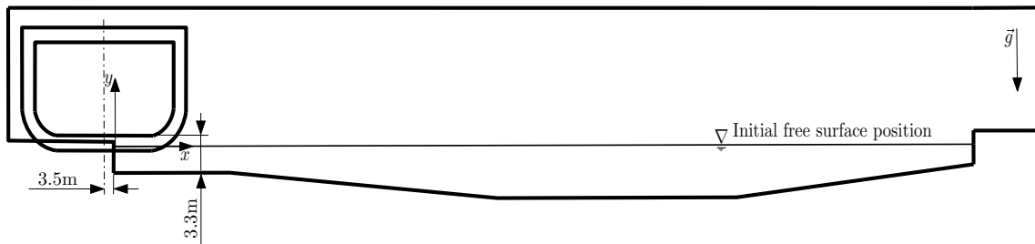
Figure 4.2: Meshes arrangement and free surface position at initial moment.
