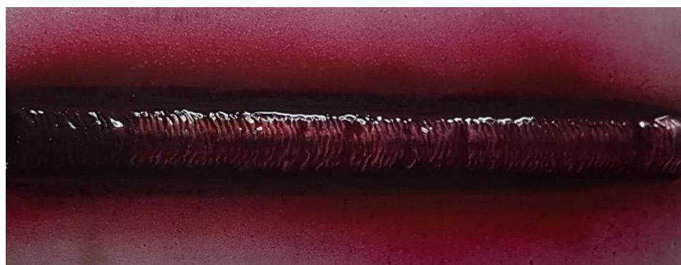
Slika 50. Uzorak A s nanesenim penetrantom - lice zavara
