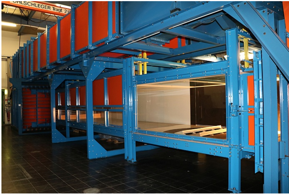
Figure 3.1: IFMHT-GUT boundary layer wind tunnel, [23].
