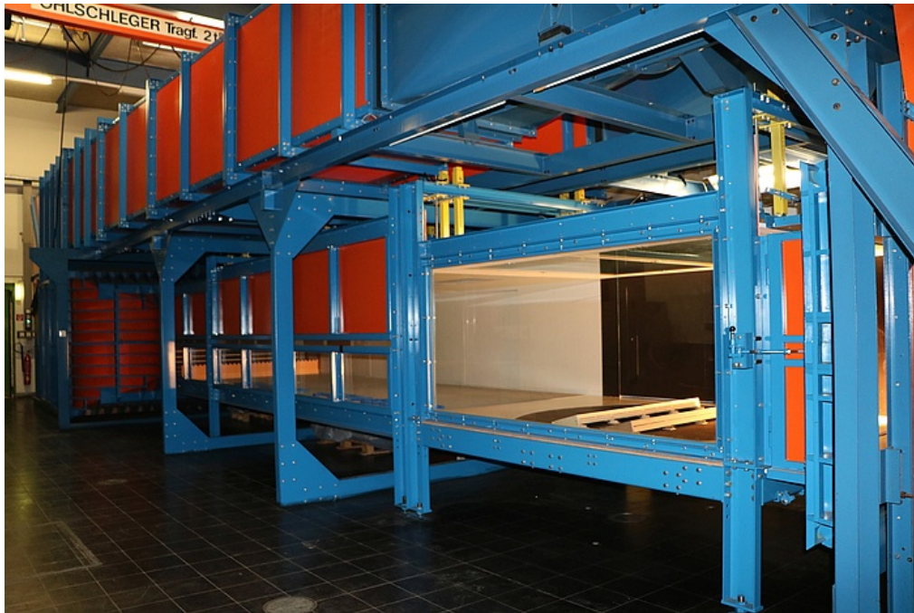
Figure 3.1: IFMHT-GUT boundary layer wind tunnel, [23].
