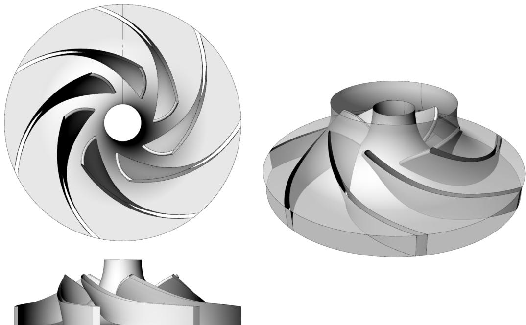
Slika 4.10: 3D model rotora,  $\epsilon_{sch} = 83 - 105^\circ$ ,  $z_{La} = 7$ ,  $e = 3.5$  mm
