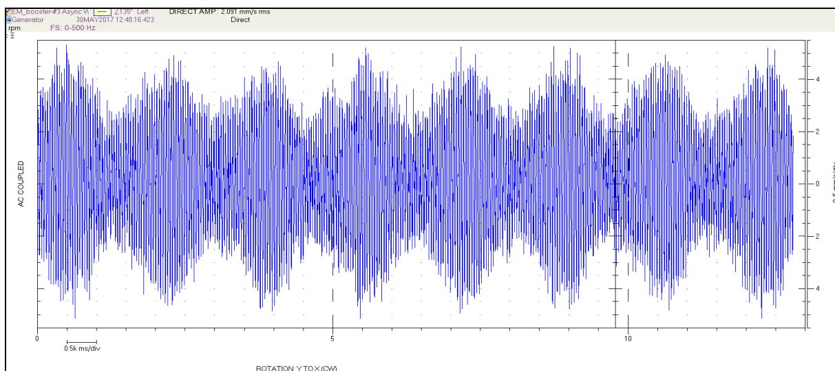
**Slika 45. Prikaz signala (timebase) Booster pumpe 2501 [19]**
