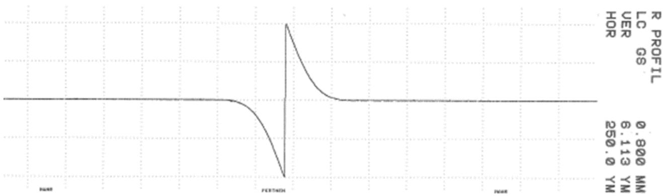
Slika 51. Simulirani profil  $Pt = 25 \mu\text{m}$
