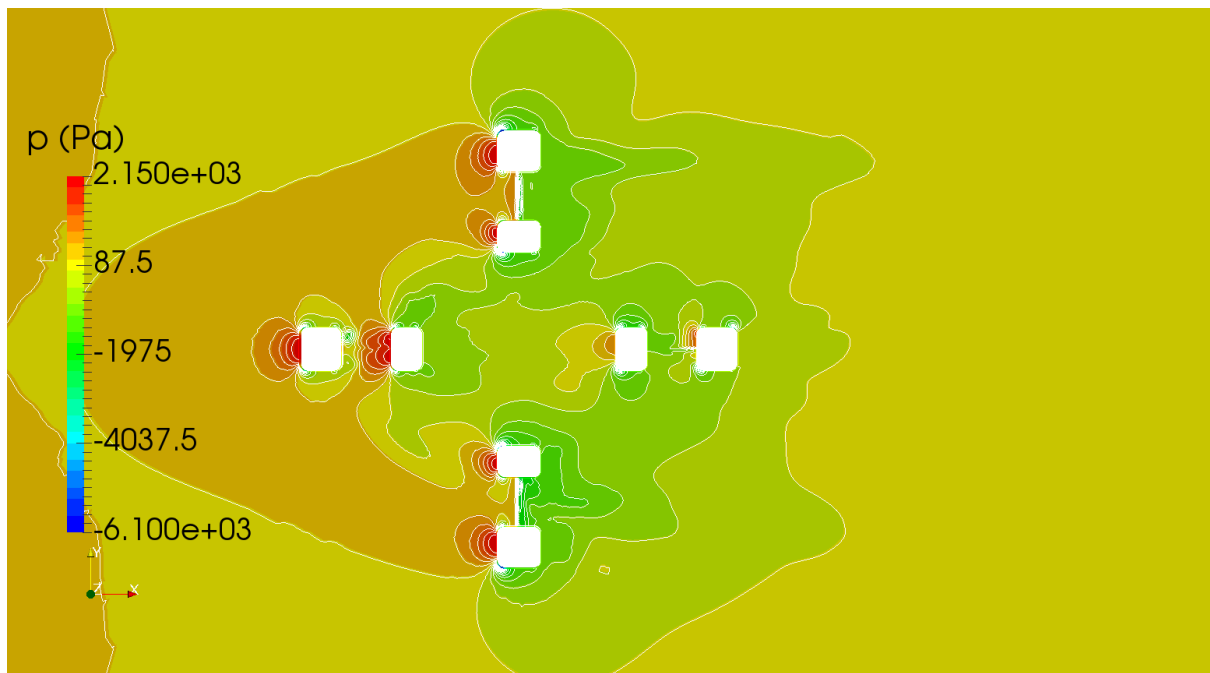
Figure 5.28: Pressure distribution on plane z = 0.085\text{m} with RANS turbulence model.
