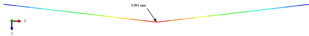
**Slika 4.6. Primjer I, Abaqus – progib  $w / \text{mm}$**
