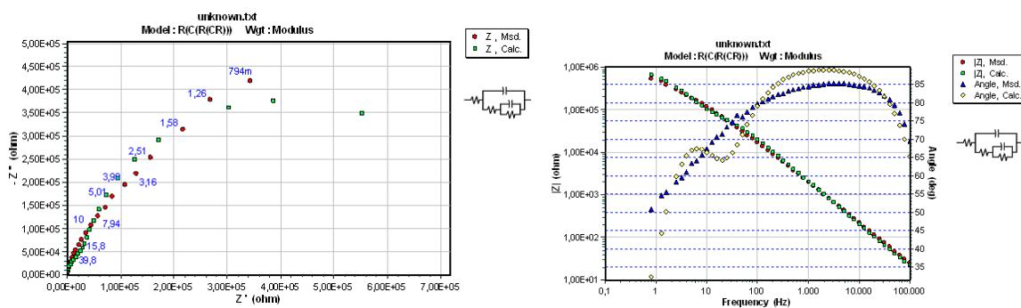
**Slika 48. Bodeov i Nyquistov dijagram za uzorak 200**
